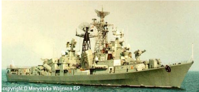
Fig. 2. Missile destroyer ORP 'Warszawa' ( D = 4\,950\text{ t} , v = 32\text{ w} ; D — displacement, v — speed of ship) [42]
