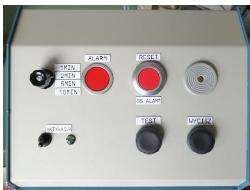
Fig. 4. Photo of Deadman Alarm Panel [4]
