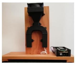
Fig. 6. Aspiration psychrometer based on digital temperature measurement
