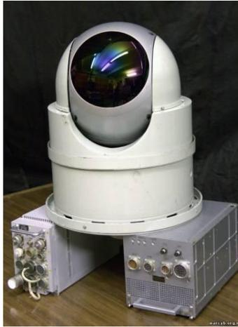
Fig. 12. Optoelectronic jamming station L370-5 [13]
