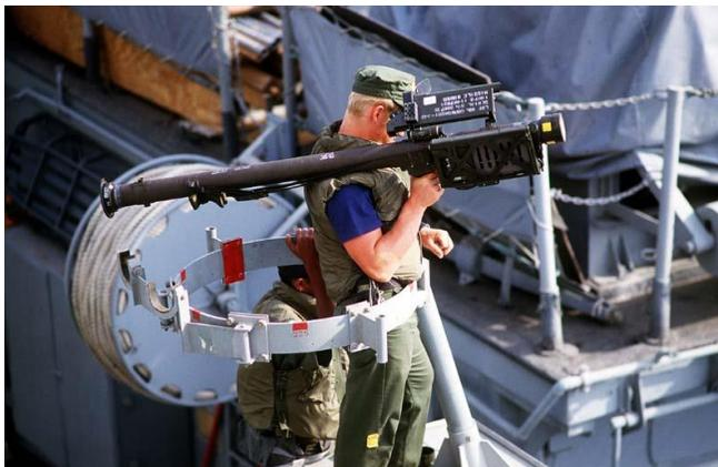
Fig. 2. The way of mounting the ring stand for the Stinger operator [20]
