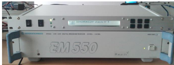
Fig. 4. Base station prototype: dedicated transmitter (top) and commercial receiver (bottom) [authors' photos]
