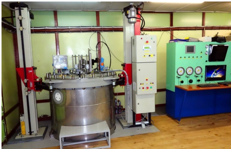
Fig. 1. Photo shows the test stand of a breathing simulator built at the Department of Underwater Works Technology Polish Naval Academy (Zakład Technologii Parc Podwodnych Akademii Marynarki Wojennej — ZTPP AMW) [from the ZTPP AMW archive]
