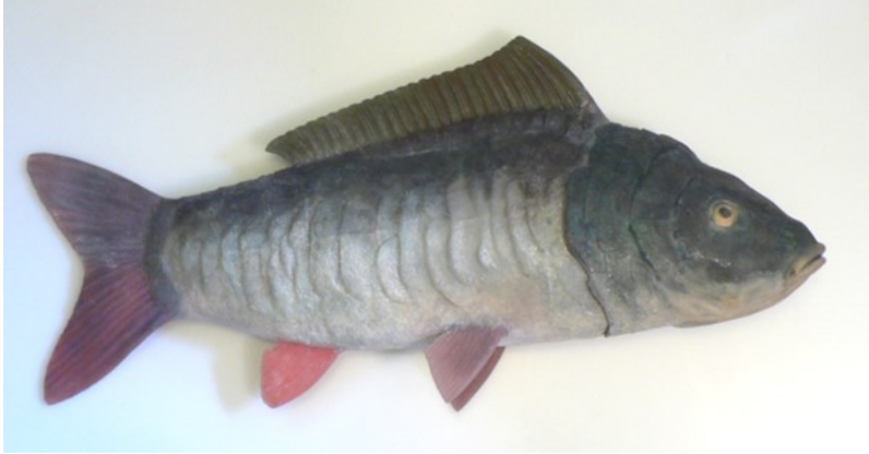
Fig. 2. Silicon coating of the CyberFish ver. 5 [7]
