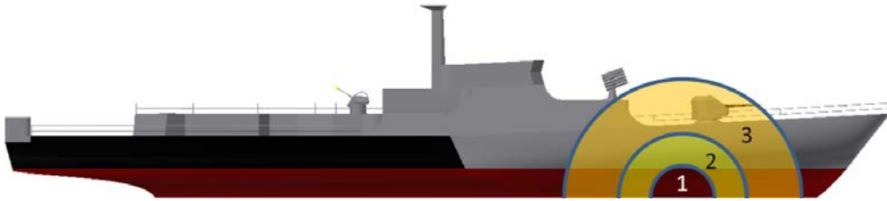
Fig. 5. Zones of destruction in a contact explosion: 1 — breach, 2 — structure bursting, 3 — zone of damage to structure and mechanisms
