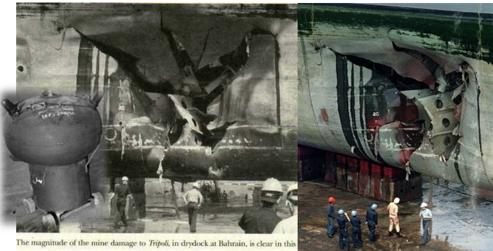
Fig. 6. Damage to the hull of the USS ‘Tripoli’ LPH-10 [17], LUGM-145 mine [18]
