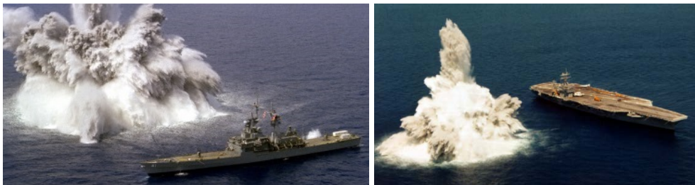
Fig. 14. An influence explosion off the beam of the guided missile cruiser USS 'Arkansas' CGN-41, 17 March, 1982 [3] and an influence explosion off the beam of the aircraft carrier USS 'Theodore Roosevelt' CVN-71, 19 September, 1987 [22]
